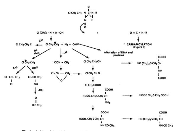
The chemical degradation of nitrosoureas leading to alkylating products, as described by Colvin et al. (1976), and some of the subsequent glutathione adducts.
